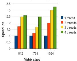
We also measured the execution time of a purely serial version of matrix multiplication with no parallel loops to measure the overhead of OpenMP on single thread performance. We found that the difference in execution time of the serial version and 1-thread OpenMP version was nearly zero in each case. Thus in this case we found no parallelization overhead over a serial version.
