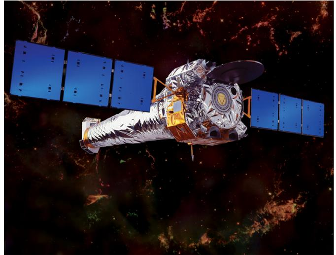
*Fig. 1: Artist's rendering of the Chandra X-ray satellite. The silverized teflon which wraps the spacecraft has degraded so it is now far less reflective than shown.*
