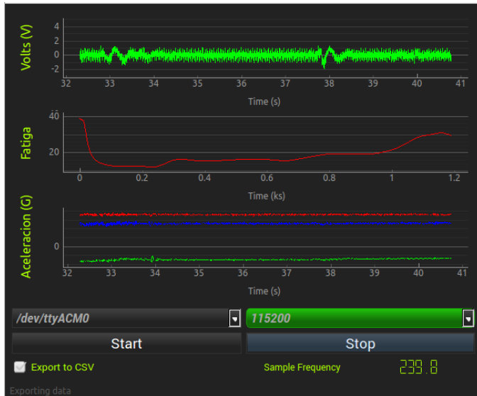
Fig. 3: Screenshot of RTGraph customized and modified to display 3 signals: an EMG signal (first panel), an estimation of the fatigue level (second panel) based on the acquired EMG signal, and three acceleration signals (third panel).
