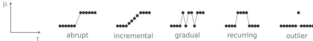
Fig. 2: Drift patterns depicted as the change of mean data values over time. Note that an outlier is not a change but noise in the data. This figure is based on [GZB<sup>+</sup>14].
