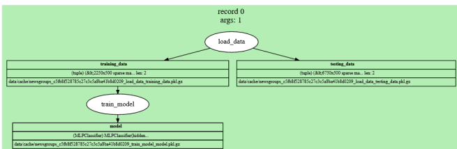
Fig. 5: Graphviz rendering of each record in more depth, showing cache file paths and artifact data types.
