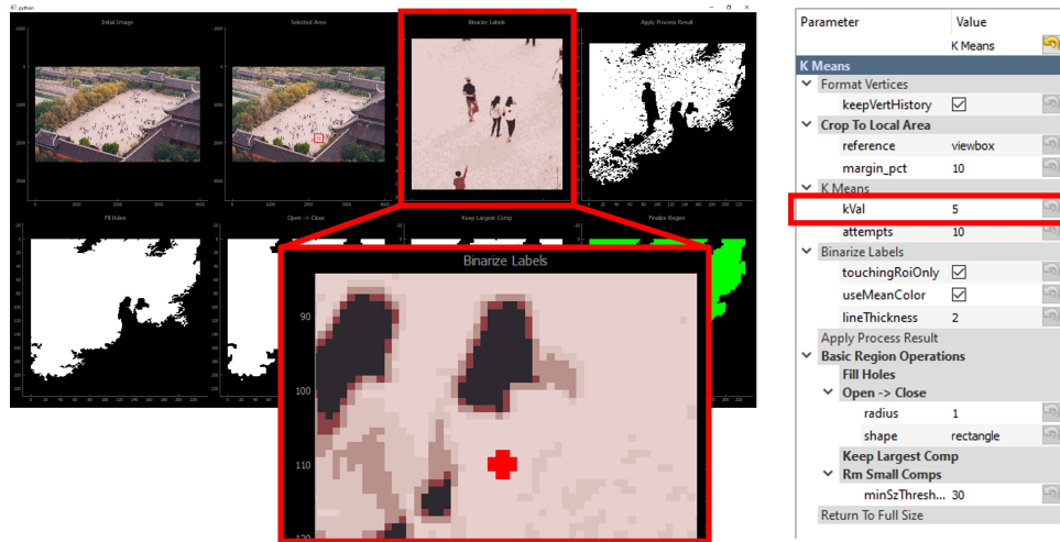
Fig. 4. Outputs of each processing stage can be quickly viewed in context after an iteration of annotating. Upon inspecting the results, it is clear the failure point is a low k value during K-means clustering and segmentation. The woman's shirt is not sufficiently distinguishable from the background palette to denote a separate entity. The red dot is an indicator of where the operator clicked during annotation.
