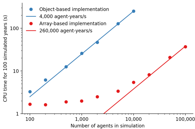
Fig. 7: Performance comparison for FPSim from an explicit loop-based approach compared to an array-based approach, showing a factor of ~70 speed improvement for large population sizes.
